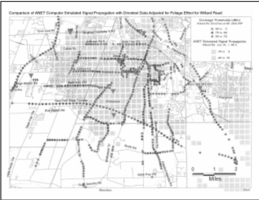
**Figure 6:** This map graphically depicts the rf-drive-test results for a proposed wireless facility. Applicants should provide color maps that have legends and are to scale.
